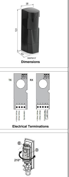
The PCB in the 900PIVOT Photocell Receiver and Transmitter can be swiveled and locked 210° to allow for versatile mountings.
